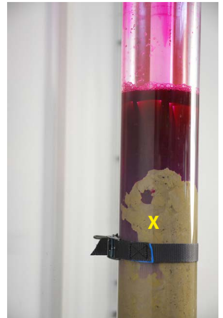
Detail product X permeable, test dye is leaking through bentonite when pumping.
