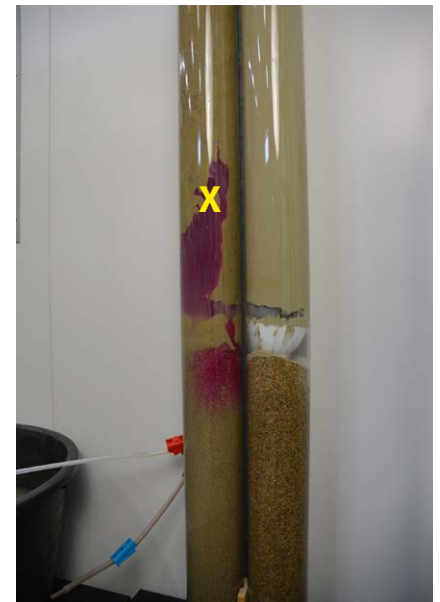
Product X test dye is leaking through bentonite when pumping.
