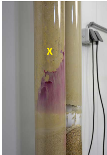
Product X test dye is leaking through bentonite when pumping.
