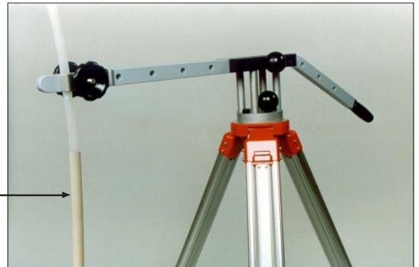
9. In an identical way a second tube can be fitted, to double the maximum output.
