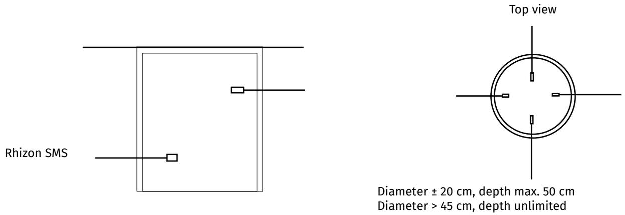
Figure 2: Rhizon SMS in PVC casing
