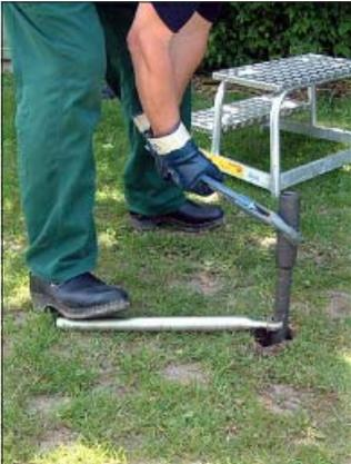
If the coupling sleeve is secured too tightly to the percussion gouge, it can be unscrewed using the pipe wrench and the catcher.
