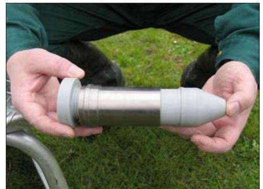
Take the thin-walled PE foil, unroll the first 20 cm and slide this over the stand to the end of the foil guide cylinder. Slide the rest of the foil over the guide cylinder.
