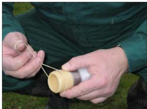
Take the extension pipe and slide the foil guide cylinder with foil and foil ring into the extension pipe.
