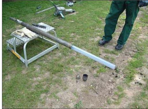
Place the core catcher in the core sampler and push the sample tube into the core sampler.
