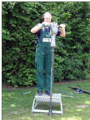
Hammer the percussion gouge into the ground. Remove the percussion hammer. Unscrew the striking pen from the coupling sleeve. If this is stuck, unscrew it using the tools supplied.
