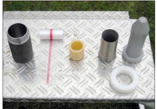
Unscrew the head from the stand and slide the guide cylinder for the foil over the long part of the stand and secure the head again. Then screw the foot into the stand and place it on a firm surface (e.g. the aluminium step-up).
