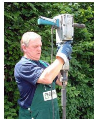
Stand on the step-up. Start the percussion hammer and keep the machine as upright as possible during hammering. If the percussion gouge "finds its own way", follow this direction with the machine. Do not force it to one side.
