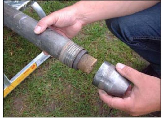
The sample can be studied immediately in the field or prepared for transport to the laboratory by closing the sample tube with protective caps.
