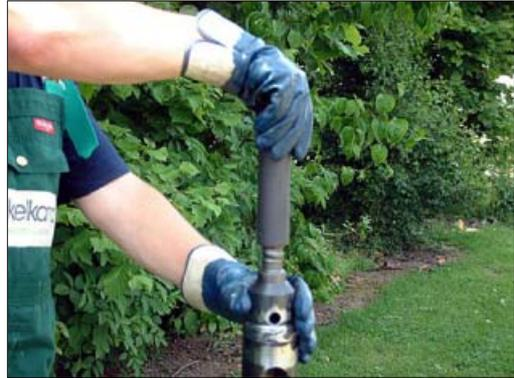
Screw the striking pen into the coupling sleeve. Note: it is left threaded. (Possibly secure with a wrench).
