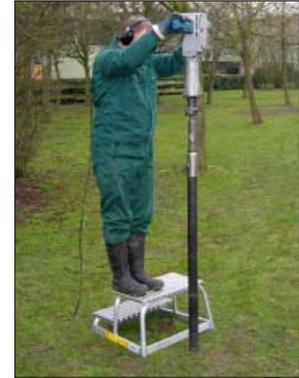
Unscrew the cutting shoe (if desired, using a wrench) and the extension pipe from the core sampler. Carefully remove the foil with sample from the core sampler.
