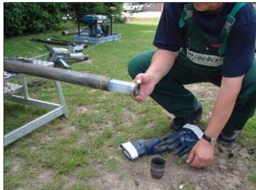
Screw the cutting shoe onto the core sampler.
