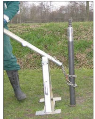
Get the next percussion gouge (with a smaller diameter than the last one).
