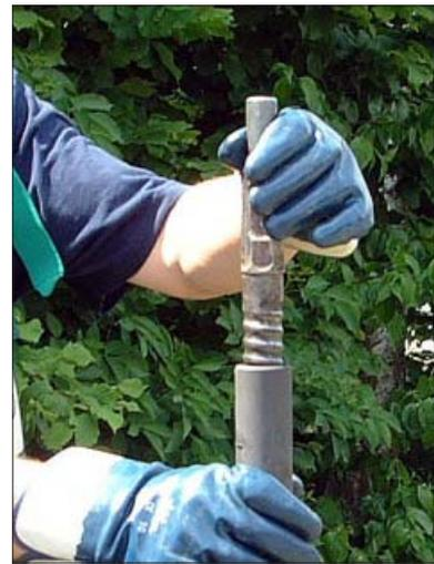
Place the aluminium step-up next to the sampling point. Insert the gouge vertically into the soil and place the percussion hammer on top. Stand on the step-up for a more ergonomic position.
