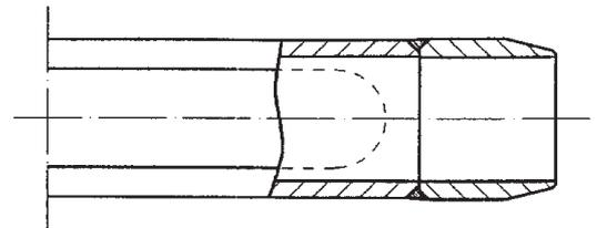
Remove the damaged cutting shoe using a saw or lathe.
