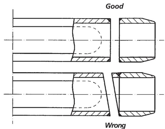
Using a grindstone, lathe or belt sander, make a slanted edge on the cut-off percussion gouge to promote the burn-in of the electrode.
