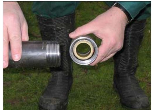
Screw it to the core sampler.
