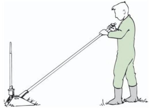
the 2-person-operated mechanical rod puller;
