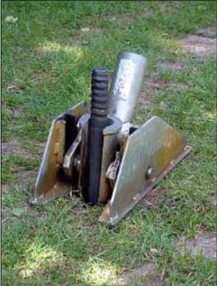
Place the universal casing and rod puller clamp on the mechanical rod puller and then place the clamping jaw in the casing and rod puller clamp. Check whether the filling ring has been fitted.
