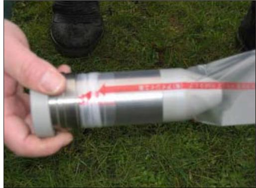
Use the slide ring to press the foil compacter onto the metal foil guide cylinder.
