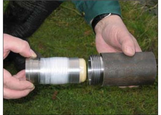
Now screw the cutting shoe to the extension pipe.
