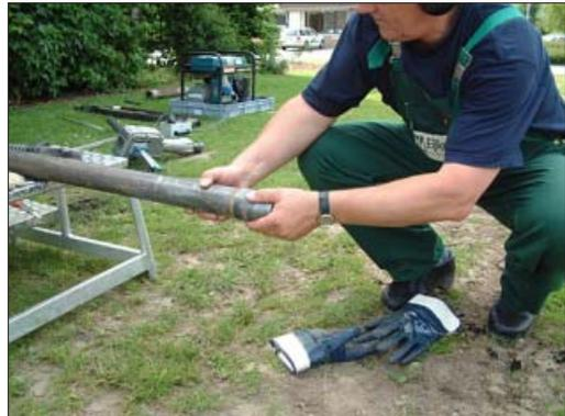
Then screw a coupling sleeve on the core sampler and screw a striking pen into the coupling sleeve (see page 3). Place the step-up and place the percussion hammer on the core sampler and hammer it vertically into the ground. When the core sampler is at the right depth, it can be pulled out in the same way as the percussion gouges (see page 5).
