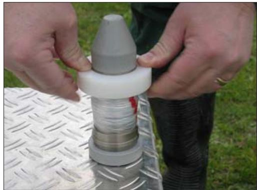
Unscrew the foot from the stand and remove the foil guide cylinder with the foil from the stand.
