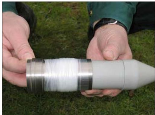
Slide the synthetic foil ring into the top of the metal foil guide cylinder.
