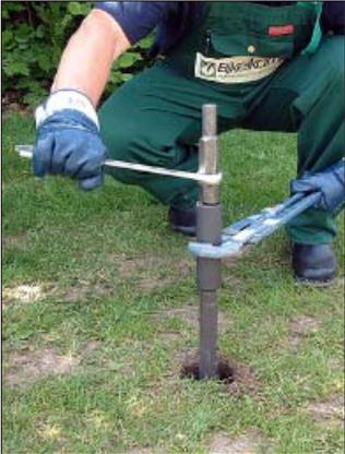
The coupling sleeve can also be unscrewed using the open ended spanner with the extension arm and the pipe wrench.
