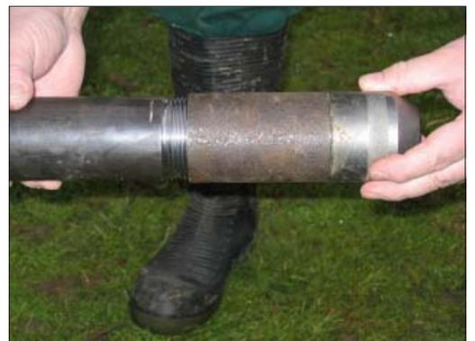
Attach a coupling sleeve and striking pen to the core sampler, place the percussion hammer and hammer the core sampler into the ground. Withdrawing it from the ground is effected as described for the percussion gouges (see page 5).
