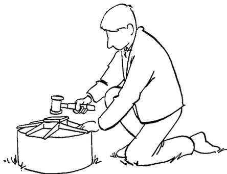
8. Fill the outer ring with water, then the inner ring, to approximately 5 - 10 cm. Start measuring immediately to determine the infiltration curve (see paragraph 3.2).
