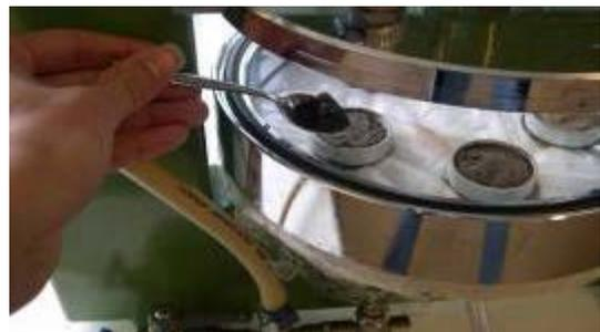
Fig. 15 Use a spoon to fill the rings with soil
