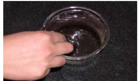
Fig. 12 Saturate the soil
