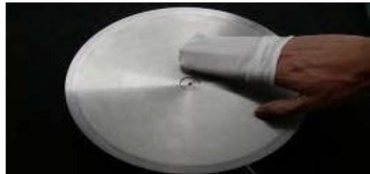
Fig. 9 Clean the base plate with alcohol
