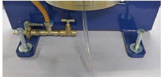
Fig. 1 Secure to a table with bolts
