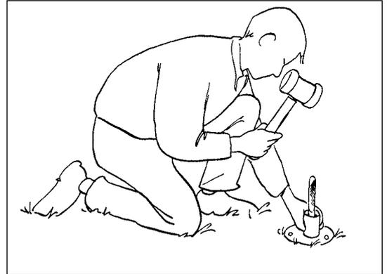
4. Remove the guide cylinder after the hole has been made. Use the spatula to dig out the hammering head to far below the sample ring.
