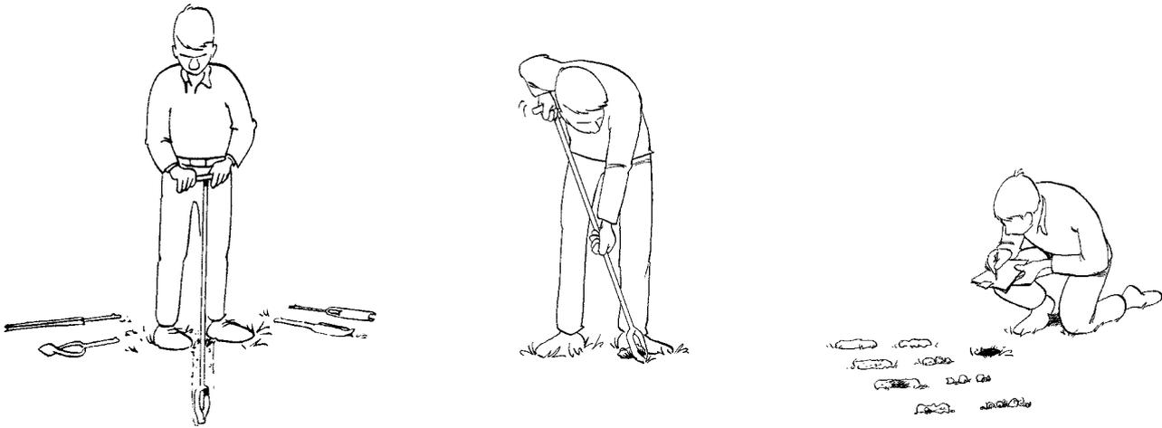
1. Hold the Edelman auger by its handle and rest it on the ground. Using some pressure, rotate the auger clockwise into the soil. After approximately  $2\frac{1}{4}$  full turns (of  $360^\circ$ ) the auger will have bored itself 10 cm into the ground. The auger will then be filled up to the bracket with slightly disturbed soil material. Dependent on the type of soil it requires more or less turns to fill the auger.
