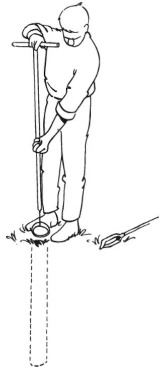
*The cutting shoe is removed from the borehole.*
