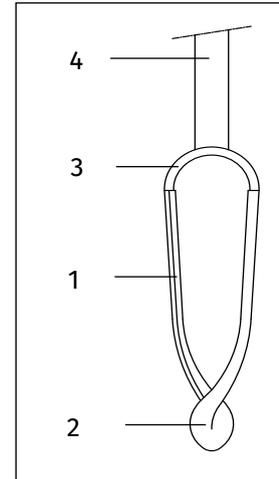
The Edelman combination type auger's diameter (measured diagonally between the blades at the broadest part of the auger body) measures 7 cm, the blades measure 35 mm in width. This permits a good hold of moderately cohesive soils, while cohesive soils can easily be removed.
