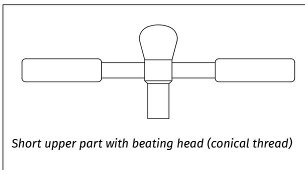
The gouge auger's operational depth measures 100 cm and has a 30-mm diameter (compare the single gouge auger for hard soils in paragraph 1.3). The upper part with beating head measures 10 cm to ensure a proper operating position and stability.
