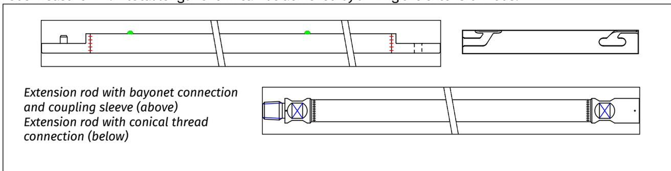
The tail ends of the extension rods are half-cylindrical and are fitted with either an eye or a pin. The eye and the pin lock into each other and are secured by a coupling sleeve. The extension rods with conical thread connections can be attached using a spanner.
