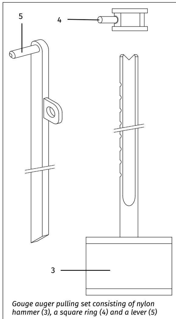
The gouge auger pulling set consists of a lever (5), a square ring (4) and a nylon hammer (3). The lever is a metal bar with an eye and a pin. One end of the bar is slanted to allow removal of the sample. The square ring has a pin welded onto it at a 45° angle. The ring is slid over the hammer handle and caught in an indentation, the eye on the lever is fitted over the pin and the lever is now in position to withdraw the gouge auger (see paragraph 5.3).
