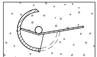
7. Upon withdrawal, lay the sampler flat on the ground, the blade on top of the gouge. Turning the blade a half circle in a horizontal position will clean the gouge, presenting a hardly disturbed sample laid out on the blade.
