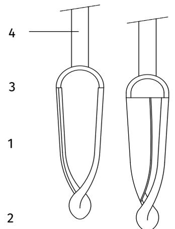
Edelman auger combination type (left) and coarse sand type (right).
