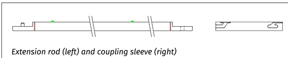
Extension rod (left) and coupling sleeve (right)
