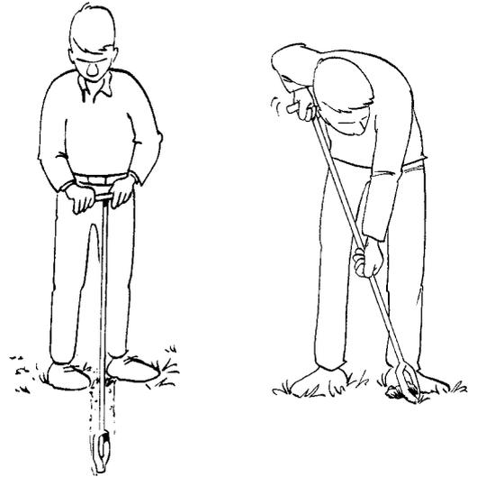
3. To obtain the sample, rotate the auger 360° clockwise without pushing down. To withdraw the auger after sampling, hoist it while gently rotating the auger. This will prevent loss of sample material. Keep your back straight and your knees bent to prevent injuries.
