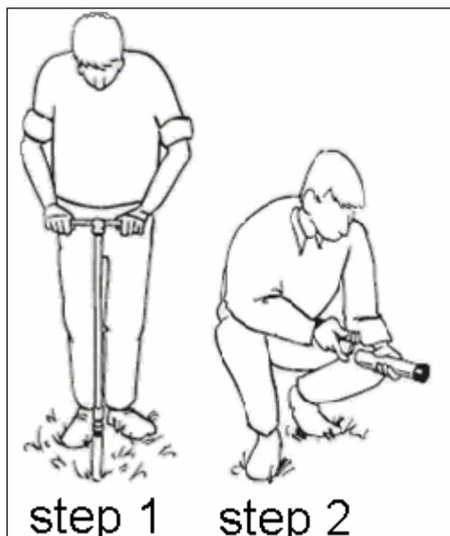
**Figure 4:** Surface sampling. Step 1-Push the core apparatus with sample core in the soil and take the sample from the soil. Step 2-Add the filling blocks in the sample tube and cap the sample tube.
